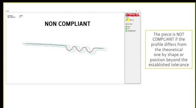
**“Before the implementation of the system, a manual measurement was made on random samples using a jig tool, which took at least two minutes to check the whole surface. With the SmartRay sensor it takes 5 seconds to automatically check the surface, resulting in 96% of time saved for a single check. In addition it is now possible to perform the inspection on 100% of production”.**
